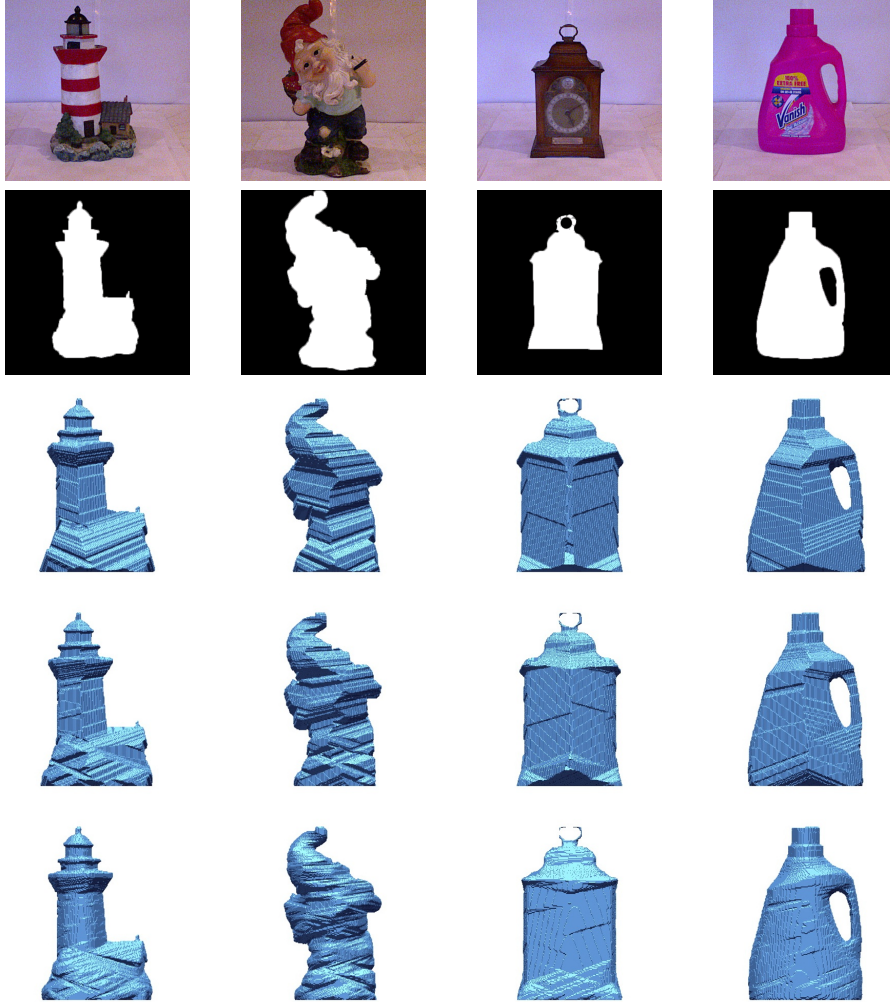
Figure 5: Shape from silhouette reconstruction using the likelihood \overline{\text{lik}}(\mathbf{x}) (modelled with \mathbf{x} \in \mathbb{R}^3 ). From top to bottom: original objects, one silhouette, reconstruction from respectively 3, 6 and 36 camera views (i.e. silhouettes).
